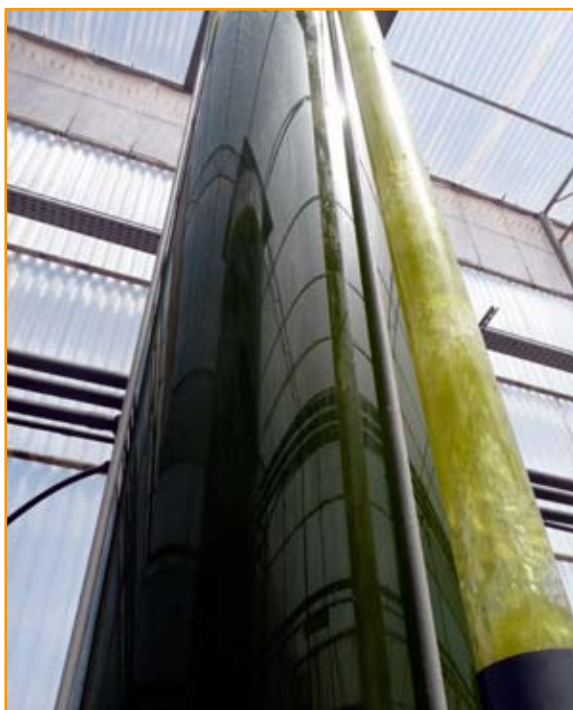
Pilot scale production of the lipogenic microalgae Nannochloopsis in tubular photobioreactor. Photography courtesy of Marine Biotechnology Centre, University of Las Palmas de Gran Canaria - National Algae Bank.
