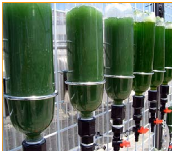
Cultivation of lipogenic microalgae in small photobioreactors (Almeida et al., 2010). Photography courtesy of Marine Biotechnology Centre, University of Las Palmas de Gran Canaria - National Algae Bank.
