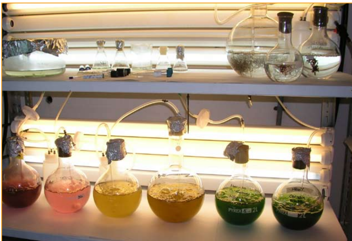
Microalgae cultures under controlled temperature, radiation and photoperiod.
