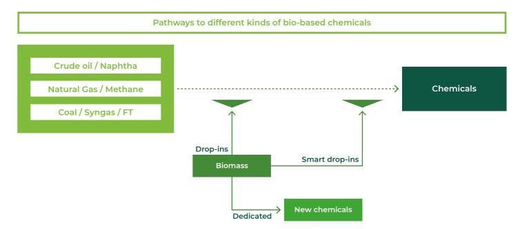
Figure 8: Schematic differentiation of the pathways of drop-in, smart drop-in, and specific innovative bioproducts (Source: RoadToBio)<sup>4]</sup>.
